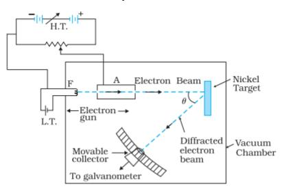
by applying suitable potential/voltage from a high voltage power supply (H.T. or battery). They are made to pass through a cylinder with fine holes along its axis, producing a fine collimated beam.
